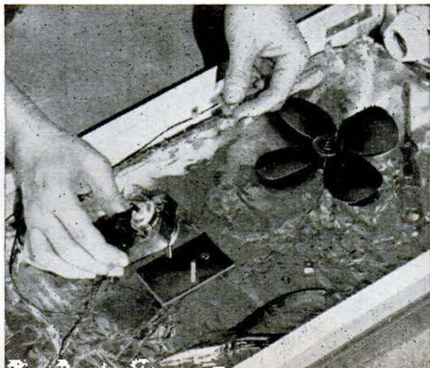
FAN IS CUSHION-MOUNTED on rubber tape or piece of inner tube after foil is in place. Notice how wires separate to front and rear.
